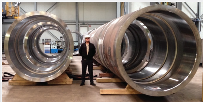
84" HYDRA-LOK™ Double Groove Sleeves (Machined)
