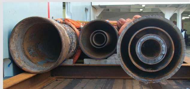
Single, triple & quadruple subsea well casings cut configurations
