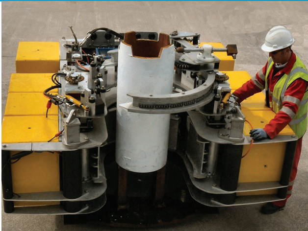
12"-24" External Cutting Manipulator Castellated cut made around the circumference of a 24" tubular
