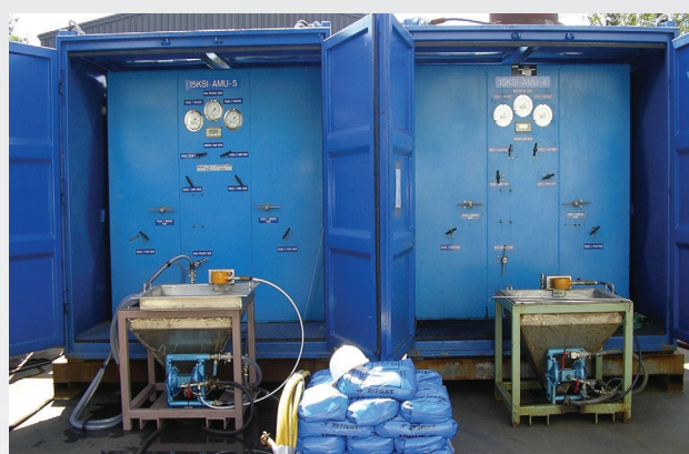
1000 bar containerised Abrasive Mixer Units (AMU) with grit-loading hoppers
