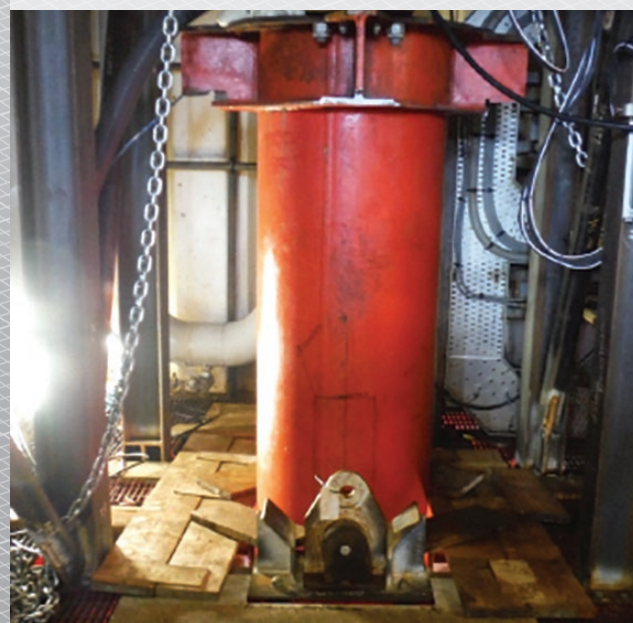
Caisson Assembly lowered into Support Pinning Frame
