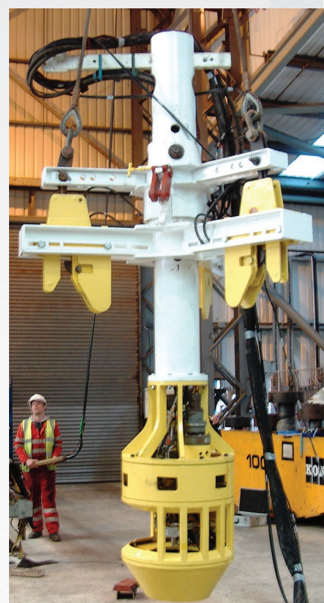
42" to 72" ICM Pile Cutting Tool Configurations
