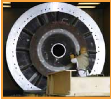
AHTS Winch Drum
