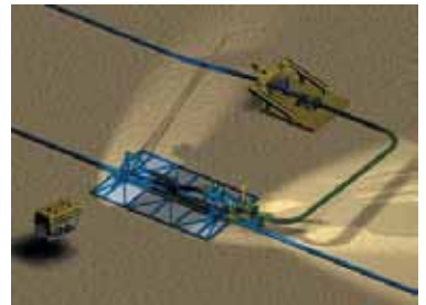
After the ROV actuates and tests the Collet Connectors, the running tools are retrieved and the tie-in is complete.
