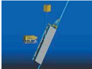
An ROV deploys the mud mats after the sled clears the stinger. A buoyancy module provides a righting moment to help the sled land upright.
