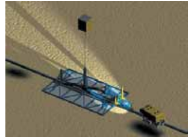
The ROV releases the buoyancy module, and sled installation is complete.
