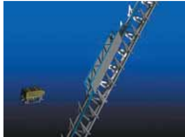
The Mid-Line Tie-In Sled is installed as an integral part of the pipeline during the S-lay or J-lay operation.
