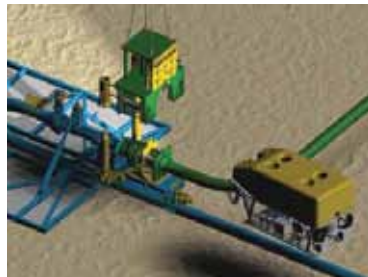
The jumper with Collet Connectors is landed, with one end on the sled porch and the other on a PLEM connected to the branch lines.
