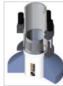
Connection made-up, hydraulic clamp assembly up, box down
