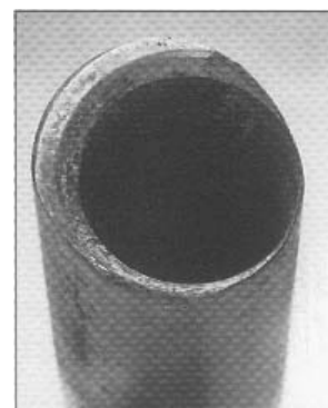
Rod coupling shows abrasive damage of metal-to-metal friction.
