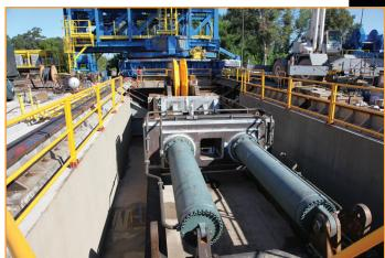
The "turn-up" sheave is a combination sheave which will accommodate either 147mm studless anchor chain or 3" diameter wire rope. The cylinders, shown here, provide the pull for the chain testing while a DC-powered, traction winch provides the pull for 3" wire rope testing.
