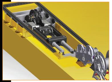
The cylinders provide up to 120 inches of dynamic testing and extreme loads while the winch allows for testing equipment at moderate loads for longer duration.
