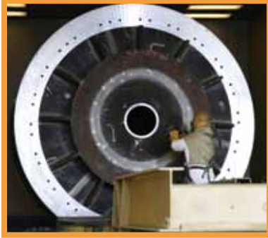
AHTS Winch Drum
