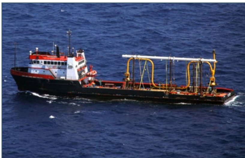
Vertical Integral Collet Connector Repair Jumper with Wye Fitting & Future Tie-in Hub in-route for deployment in the Gulf of Mexico
