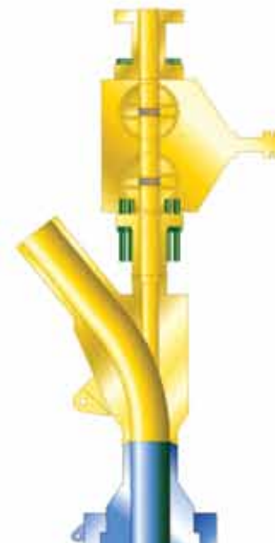
The Block and Bleed Gate Valves are closed, the Plug Installation and Removal Tool is unbolted and removed, and the Intervention Y is ready to receive the coiled tubing or wireline unit. The procedure is reversed to reinstall the Diverter Plug.
