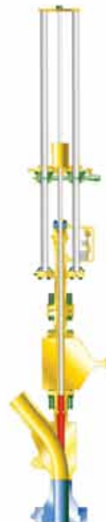
After seawater is displaced, the block-and-bleed valves are opened and the Screw-Jack Gearbox is operated to lower the Insertion/Removal Shaft to the Diverter Plug.
