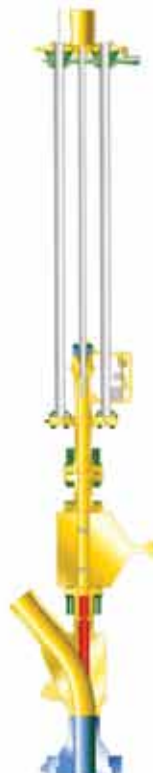
After pressure is bled off and the annulus is purged and flushed, the blind flange is removed, the Plug Installation and Removal Tool is installed, and seal integrity is tested.
