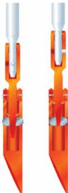
The Shaft engages the Actuator Bolt in the Diverter Plug. Shaft rotation raises the Actuator Bolt, retracting the Locking Dogs and releasing the Diverter Plug for removal
