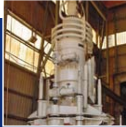
LMRP with FlexLoops and FlexJoint® installed
