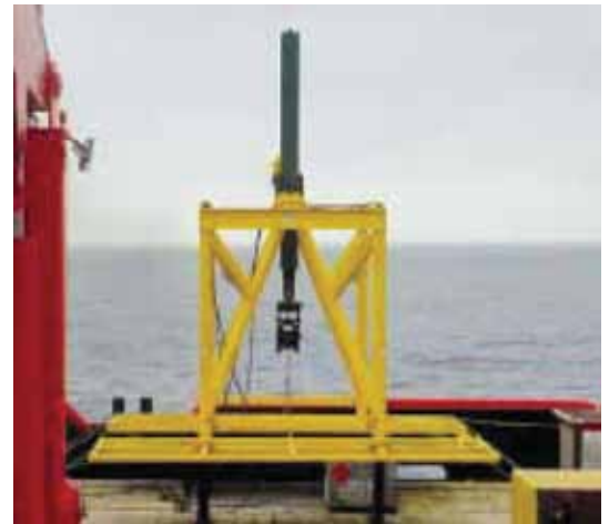
Diverless Pipeline Lift Frame on deck, ready for deployment
