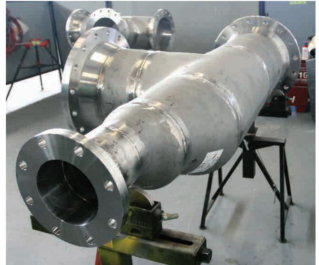
High alloy process piping MGTAW welds
