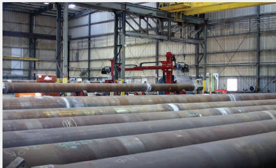
Large diameter and heavy wall fabrication of carbon steel pull tubes. Final length 165 feet long with C class fatigue sensitive welds.
